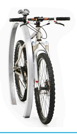
The Horizon Bike Rack is a modernized bike rack design with the capacity of two bikes. The frame is 2" square x 11 gauge steel tubing and has the perfect balance of a modern design and security. Choose between a surface mount or inground mount based on your needs. The heavy duty frame is powder coated a bright color to stand out to cyclists. The Horizon Bike Rack is 37" high and 42" wide.
