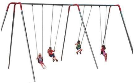
Our 10 foot Heavy Duty Modern Tripod Swings come with black cut-proof belt seats, 4/0 galvanized welded steel chain, and self-lubricating swing hangers. There are 2 seats per 10 foot section. The dimensions are as follows: 3-1/2" OD galvanized top rail, 2-3/8" OD galvanized legs, 10' installed height.
