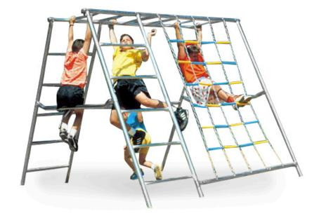
The Net Climber is constructed of galvanized steel piping with a plastic covered climbing net. The climber is 6 feet high x 7 feet square base, and the top is 2 feet wide. The sloped slides provide children a climbing challenge. Available as a portable or permanent unit, the permanent climber includes an anchor kit. Permanent climbers are required for commercial applications.
