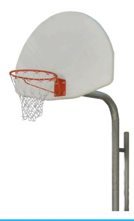
This backstop is extra rigid and comes with a 3 foot extension. The 3.5 inch OD galvanized steel bent post is reinforced with a 2-3/8 inch OD galvanized steel pipe welded 6 inches behind it. Comes complete with backboard, post, official goal, and nylon net. The Bent Post Backstop is intended for heavy use in park, school, and public settings.
