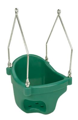
Our rotational molded infant swing seat made of polypropylene. The seat meets ASTM standards for commercial use in school and park playgrounds. The extra wide hanger is especially designed so that the seat is gravitationally correct when a child is swinging in the seat. The hanger is made of stainless steel. The dimensions are: 12" across, 11.5" front to back, leg holes 6.5" diameter, seat is 8" deep. Available in black, red, blue, yellow, and green.
